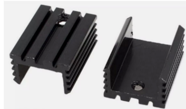
Slightly bigger heatsink for TO-92 package
